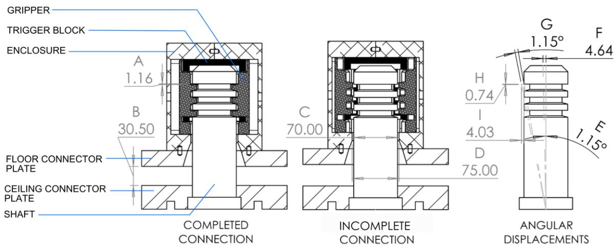
**Figure 4.** CAD analysis of functional gaps and clearances between floor and ceiling connectors for a successful connection.
