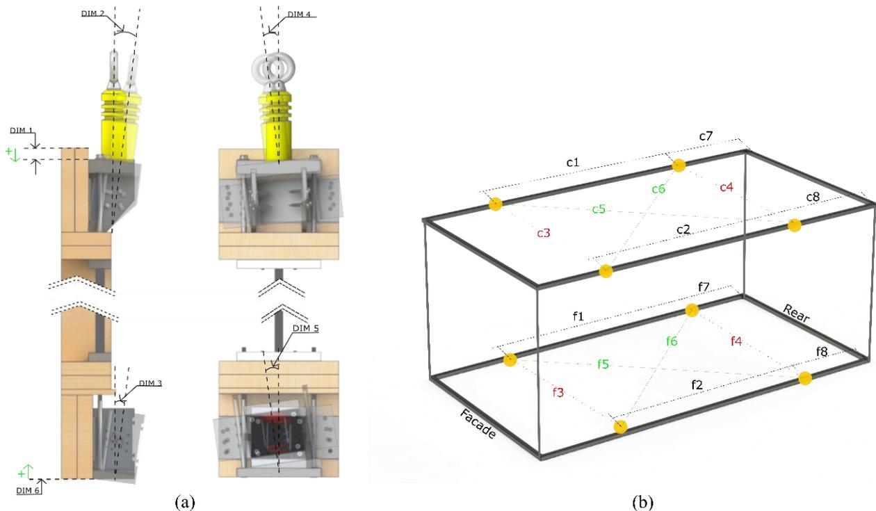
**Figure 5.** Critical dimensions for the accurate positioning of ceiling and floor connectors (a) on the vertical plane and (b) on the horizontal plane.
