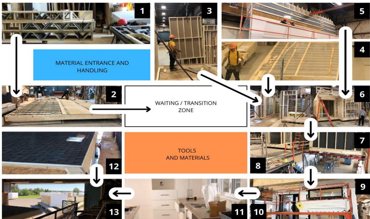
**Figure 3.** Module manufacturer of full-scale experimental project factory schematization with 13 identified workstations at specific locations.
