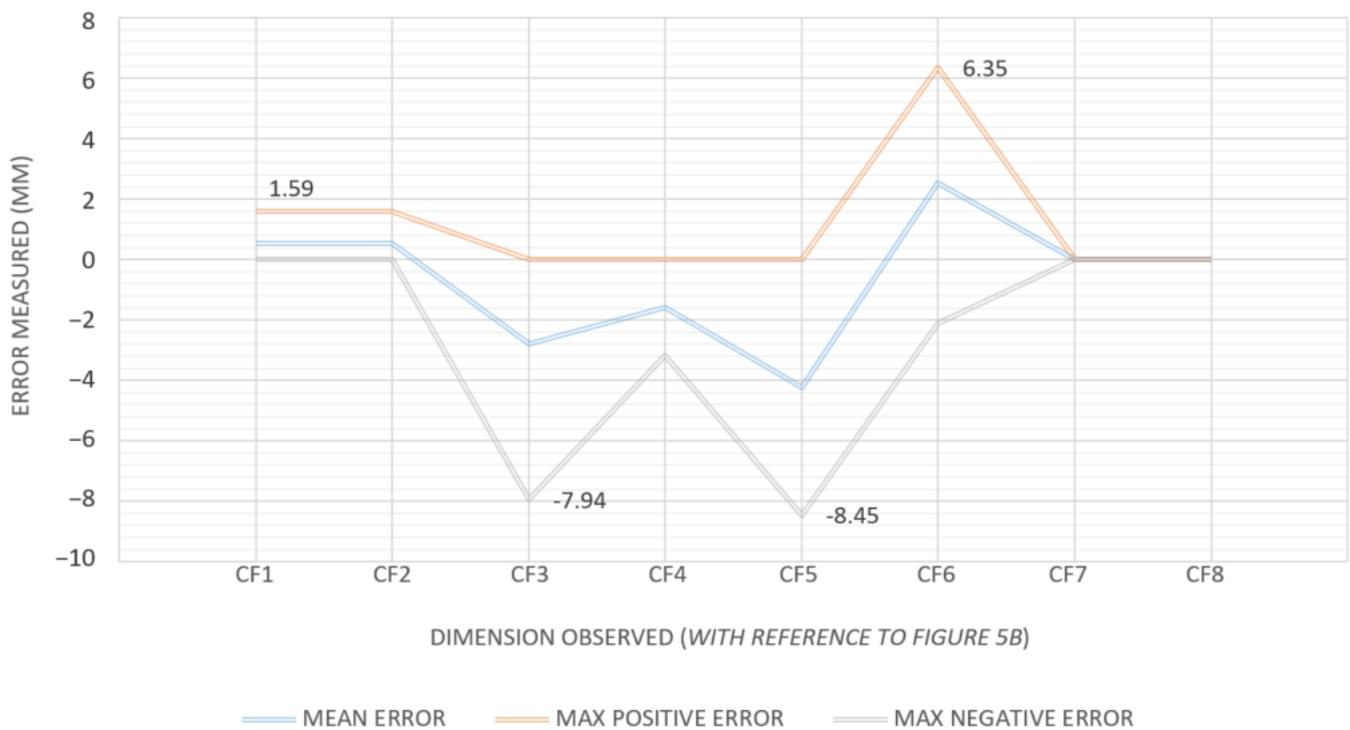
**Scheme 1.** Dimensional control for positioning the connectors, in-plane dimensions.
