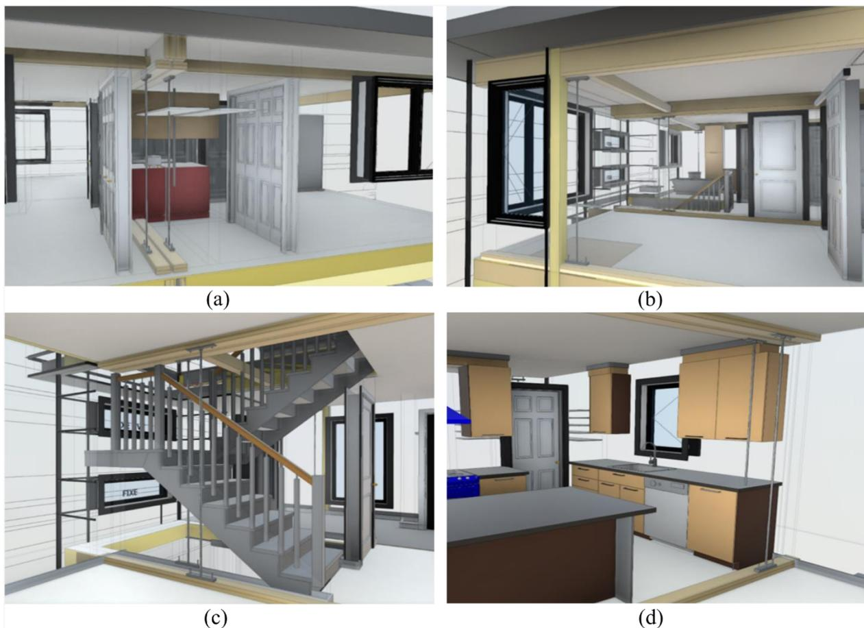
**Figure 2.** Observations and considerations of the use of an automatic connecting and lifting device in BIM modelling: (a) bedroom area, axes located in the closet; (b) bedroom area, axes located at the window limit; (c) open living room area, axes located in the open staircase; and (d) kitchen area, axes located through the countertop.
