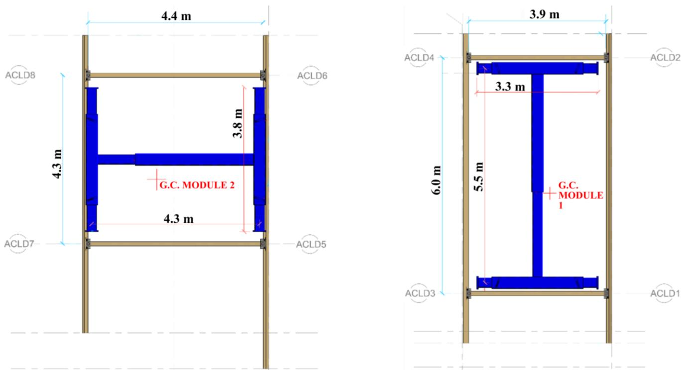
**Figure 6.** ACDs positions in the left and right modules, center of gravity, and spreader beam configurations for lifting.
