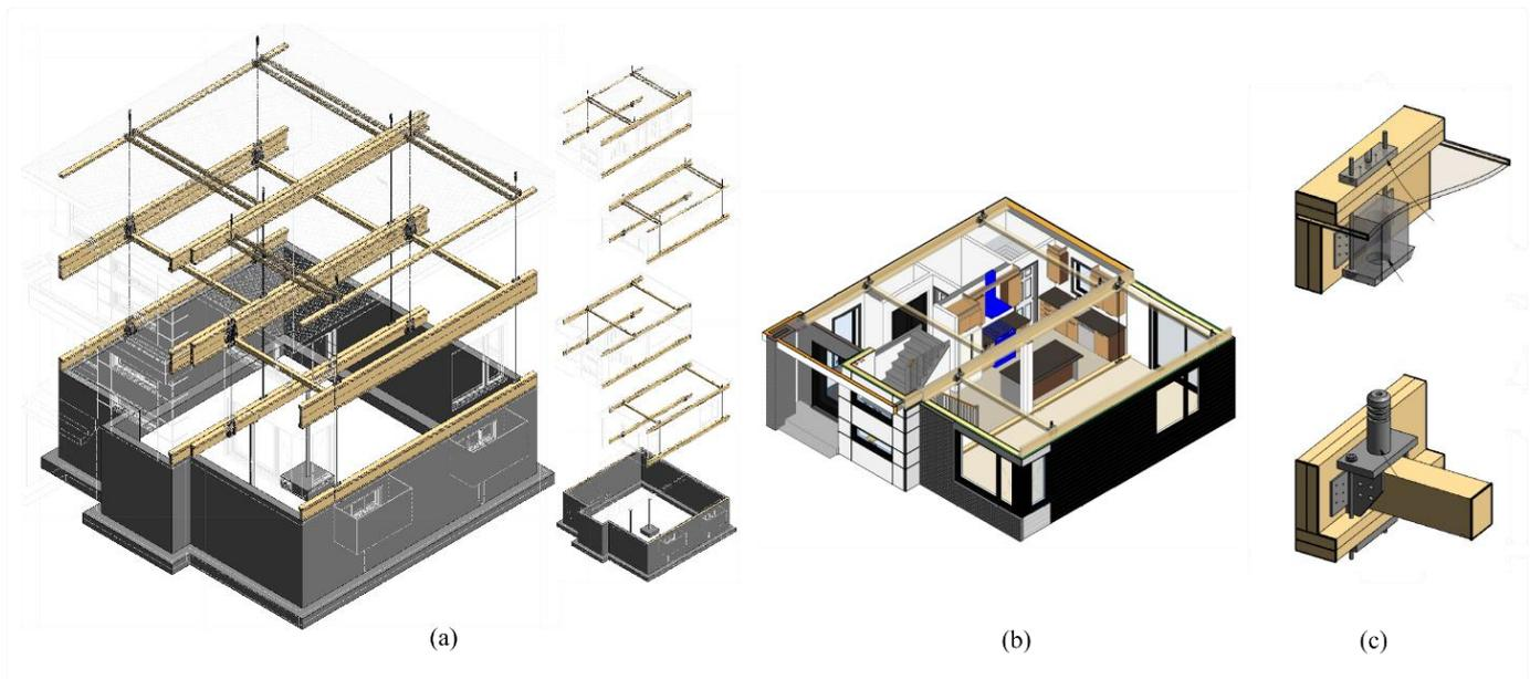
**Figure 1.** Inclusion of ACDs and lifting axes to plans: (a) structural skeleton; (b) architectural and mechanical/electrical/plumbing systems; and (c) BIM family parts for floor connector (hollowed) and ceiling connector (extruded).
