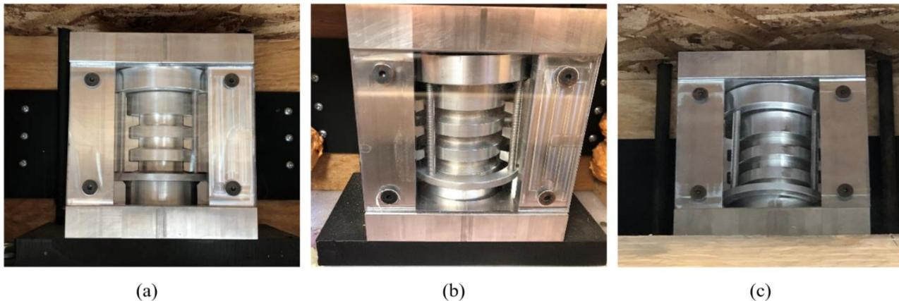
**Figure 8.** Three ACDs in the full-scale experimental project: (a) complete connection (ACD F2); (b) incomplete connection (ACD 8); and (c) incomplete connection with visual signs of interference on all the teeth (ACD F7).
