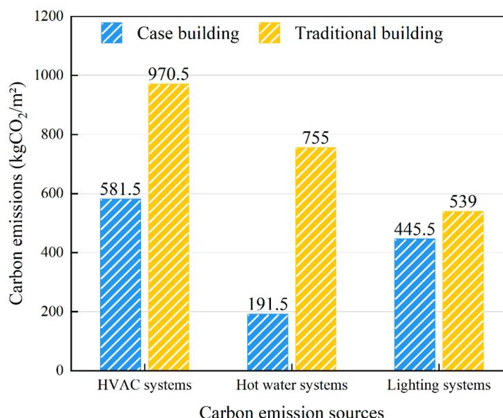
**Figure 6.** Comparison of carbon emissions at operation stage.
