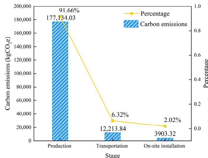
**Figure 5.** Carbon emissions distribution at the materialization stage.
