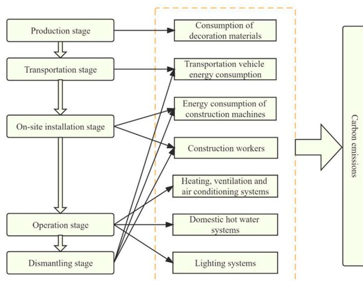
**Figure 2.** Measurement boundary for prefabricated decoration carbon emissions.
