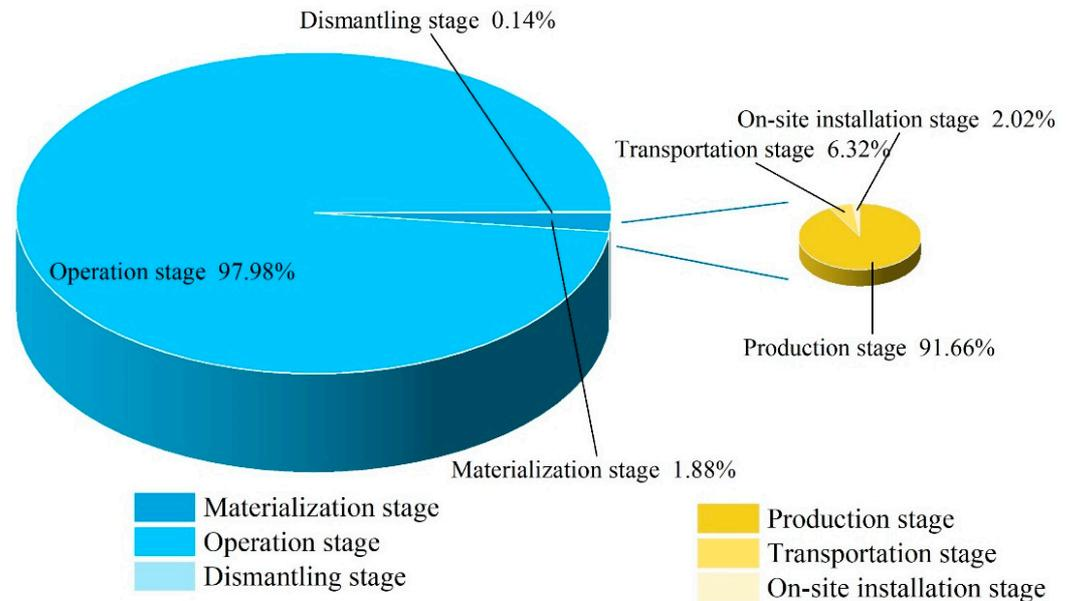
**Figure 7.** Carbon emissions percentage at each stage of the prefabricated decoration.
