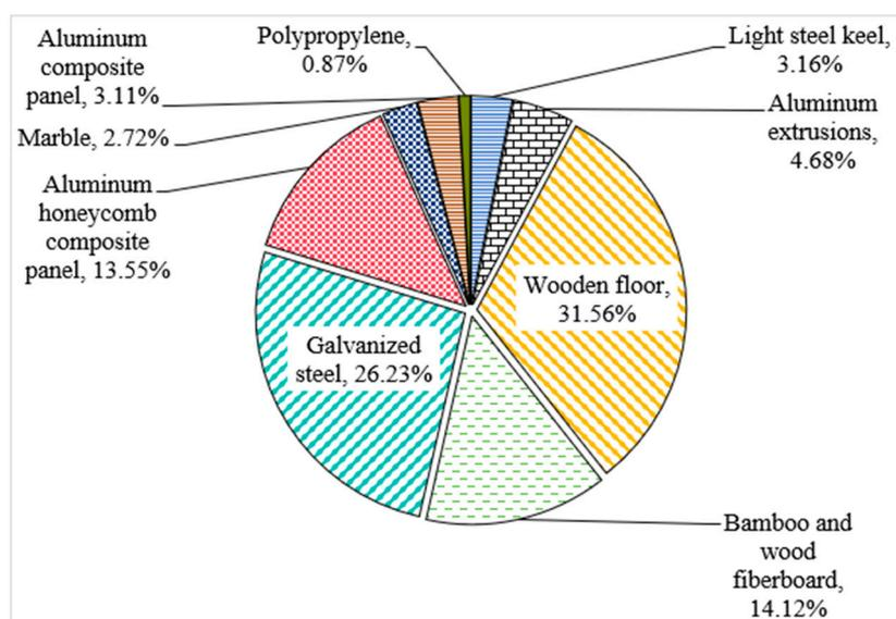
**Figure 3.** Material share of carbon emissions at the prefabricated decoration production stage.
