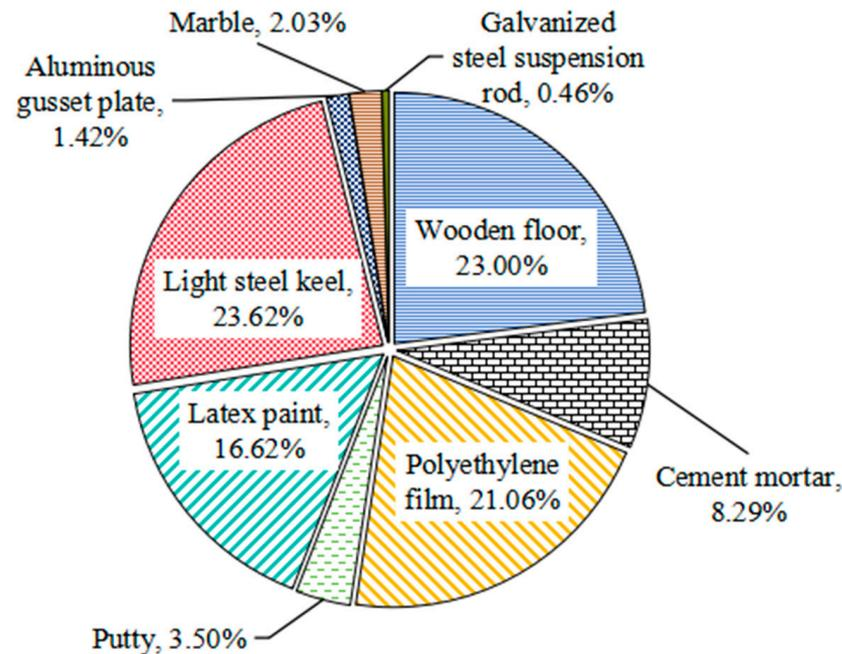
**Figure 4.** Material share of carbon emissions at the traditional decoration production stage.
