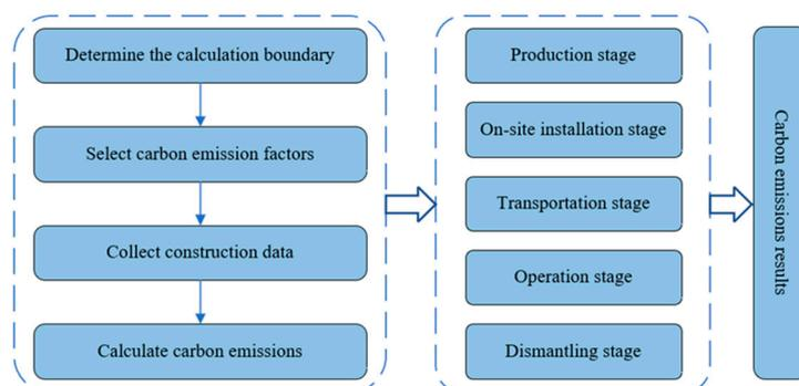
**Figure 1.** Carbon emissions measurement framework for prefabricated decoration.
