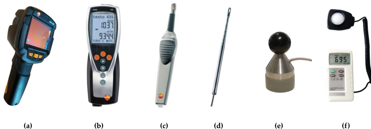
Figure 5. Instruments and measuring equipment used: (a) Testo 868 thermal imaging camera; (b) thermal transmittance flowmeter Testo 435-2; (c) humidity/temperature probe with wireless handle; (d) surface probe; hot wire probe; (e) black balloon probe; (f) luxmeter.
