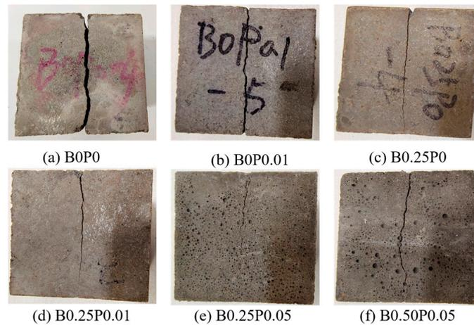
Figure 17. Typical failure modes of mortar specimens after split tensile tests.
