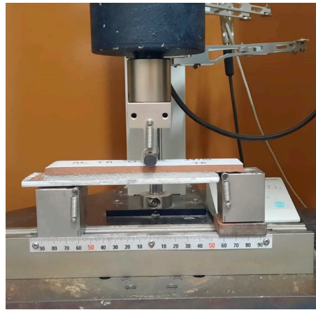
Figure 2. Mixed-mode flexure test.
