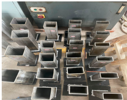
(a) Connect to flat plate and seal with silicone adhesive
