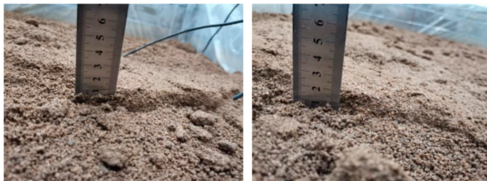
Figure 23. Maximum surface settlement of the model.
