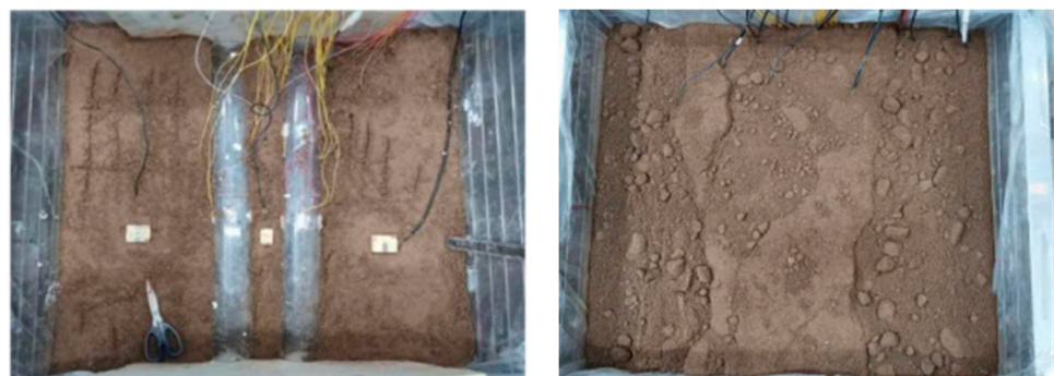
Figure 22. Surface settlement of the model.
