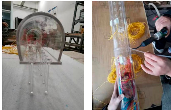
Figure 11. Tunnel–pile structure model.
