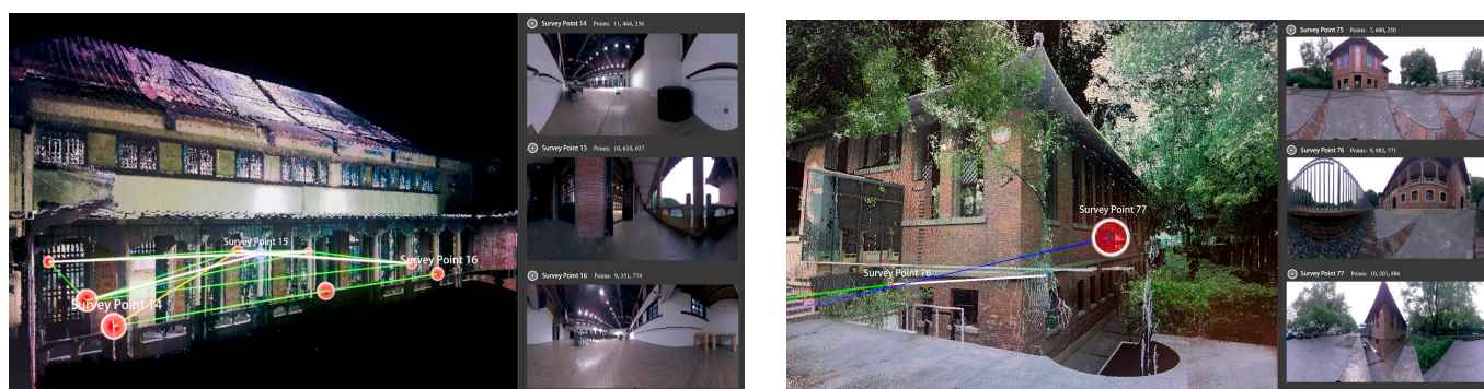
Figure 8. James Jackson Gymnasium point cloud data model at spliced measuring station 1 (measuring points 1–15) and the scanning panorama corresponding to each measuring point, and the right text part is the total number of point cloud data points contained in the measuring point (left); the scanning panorama corresponding to each measuring point of James Jackson Gymnasium point cloud data model at spliced measuring station 6 (measuring points 76–90), and the right text part is the total number of point cloud data points contained in the measuring point (right).
