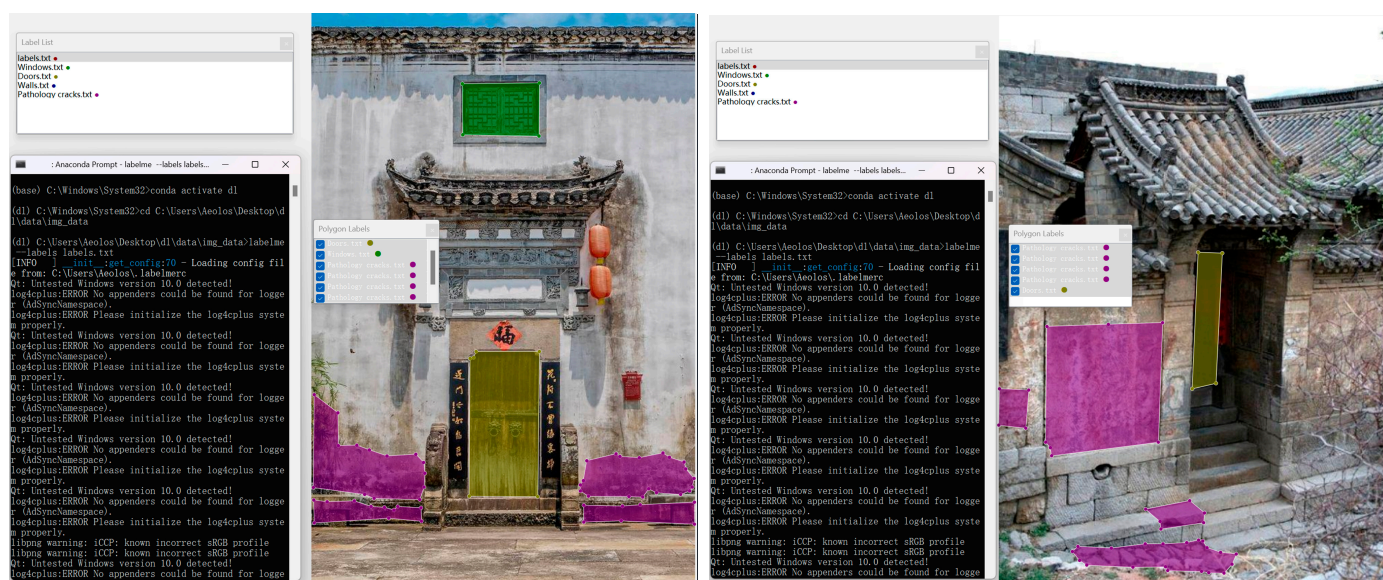
Figure 9. Architectural heritage pathology cracks training dataset. In order to enhance recognition accuracy, annotated images are predefined and displayed within a white box. Green signifies the window category, yellow signifies another category, purple signifies architectural heritage pathology cracks, and the portion within the black box represents the running code.
