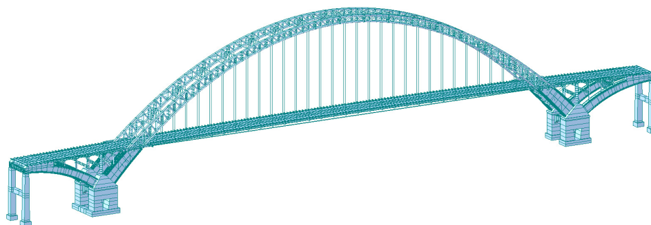
Figure 3. Finite element model of Hejiang Yangtze River Highway Bridge.
