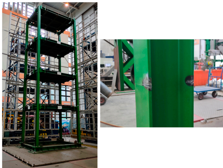
Figure 9. The photograph of the full-scale specimen and the cut column on the shaking table.
