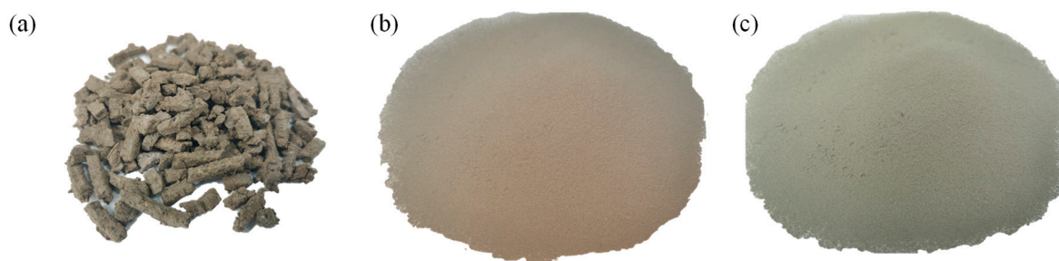
Figure 1. Morphologies of raw materials: (a) sewage sludge; (b) CFA; and (c) CCFA.
