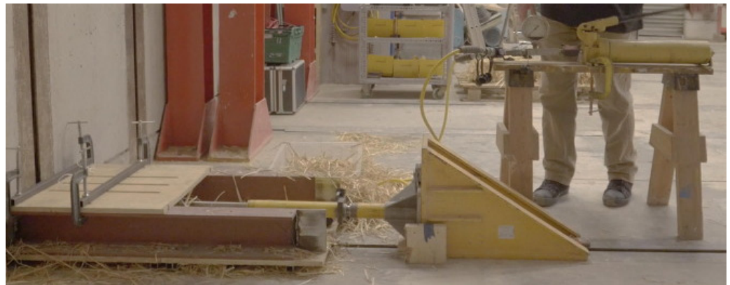
Figure 6. Production of oriented prototype straw bales.
