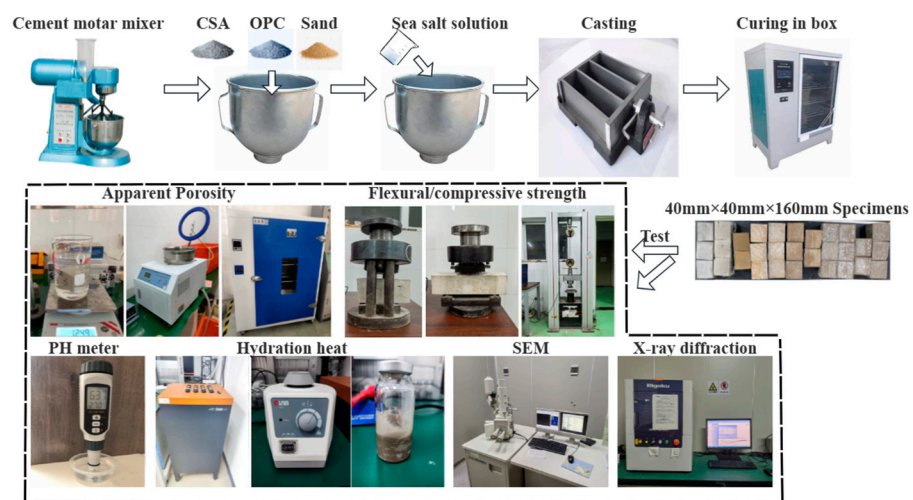
Figure 2. The manufacturing process and experimental method of CSA.
