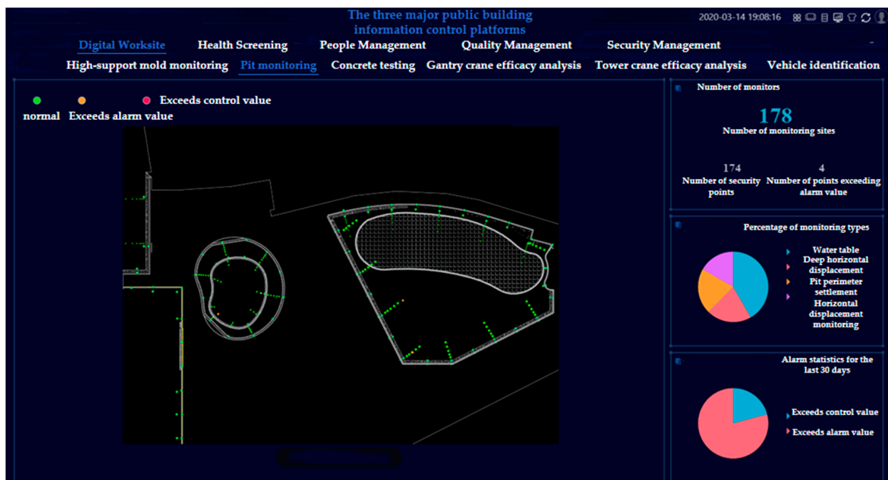
Figure 6. Twin platform for foundation pit safety monitoring.
