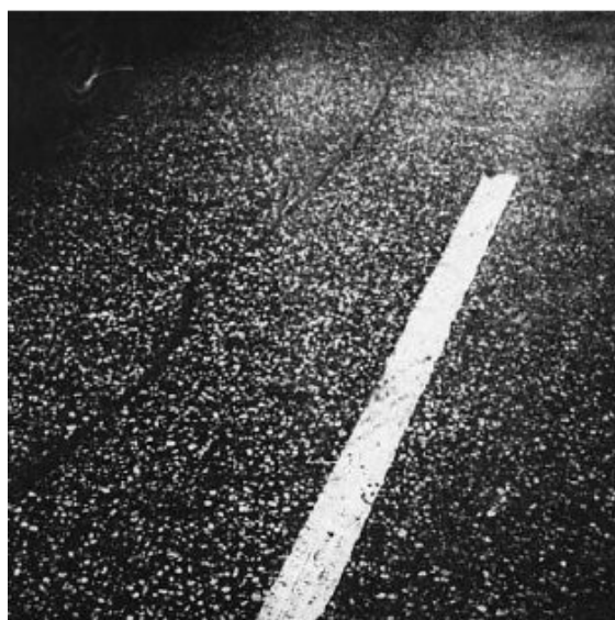
Figure 5. Visibility improvement of pavement surfaces with WG particles.
