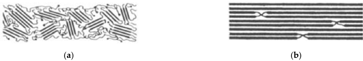
Figure 1. Micro-structure of fiber, (a) normal polyethylene with low molecular orientation, (b) Ultra-High Molecular Weight Polyethylene Fiber [73].
