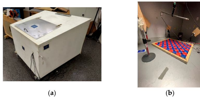
Figure 5. (a) Scaled reverberation chamber; (b) Details of scaled reverberation chamber test.
