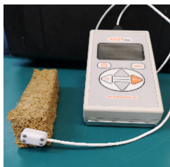
Figure 2. Thermal conductivity measurement equipment.
