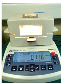
Figure 3. Process of measurement of moisture.
