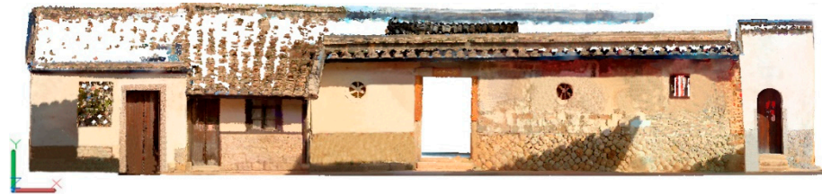
Figure 7. Point cloud front facade slice.
