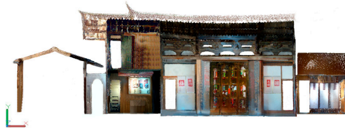
Figure 11. Point cloud transverse section slice.
