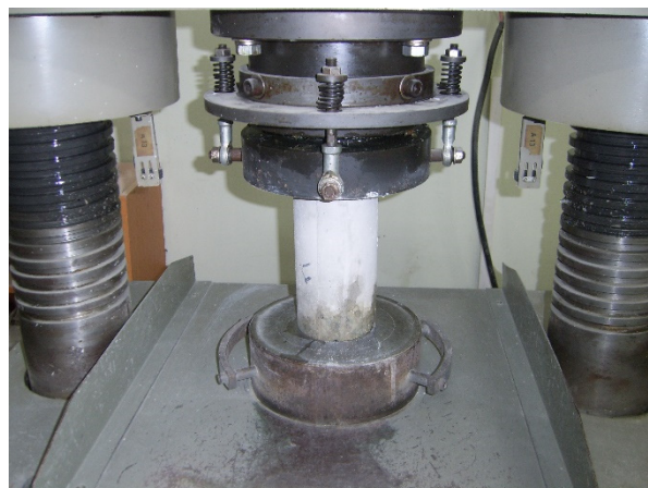
Figure 2. The compressive strength test.
