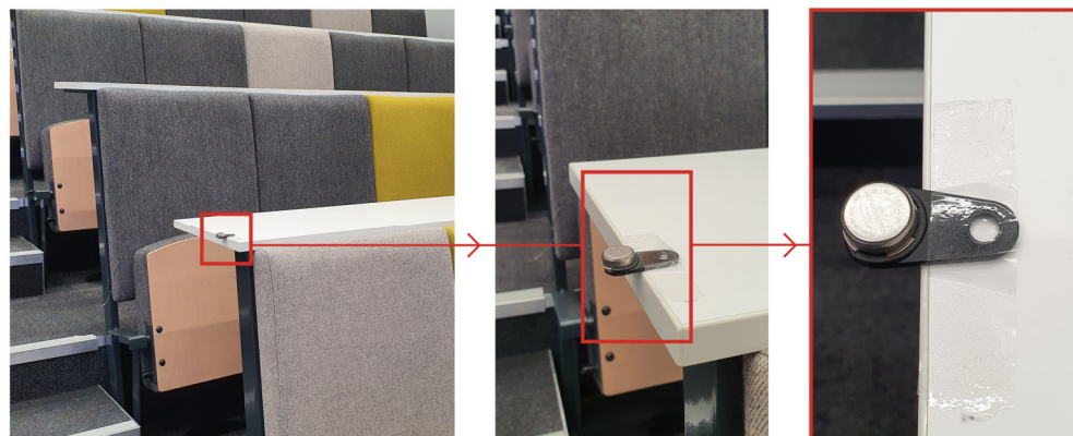
Figure 2. Photos showing how the data logger was placed during the measurement.
