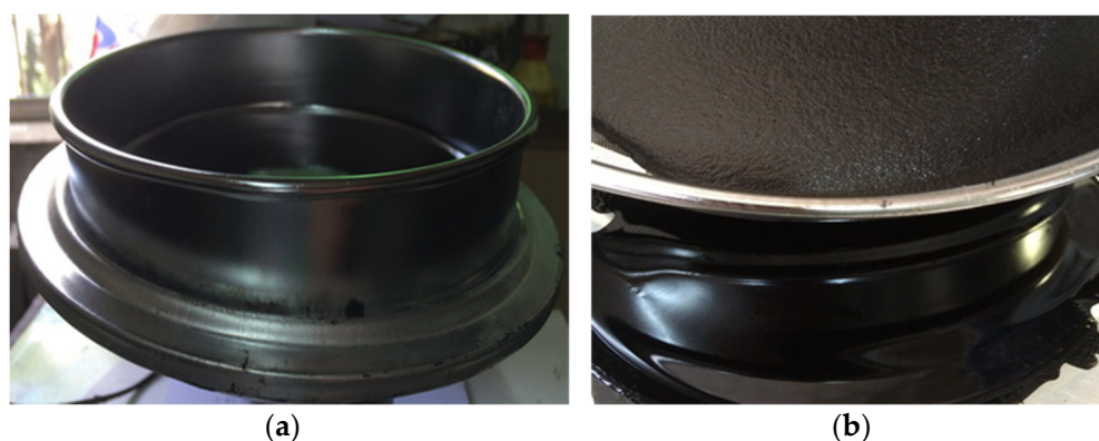
Figure 2. The separation of rubber and modified asphalt. (a) Before separation. (b) After separation.
