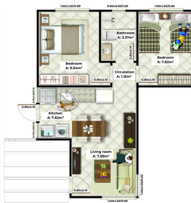
Figure 1. House floor design plan of the residential unit studied. Source: Adapted from Martins et al. [22].
