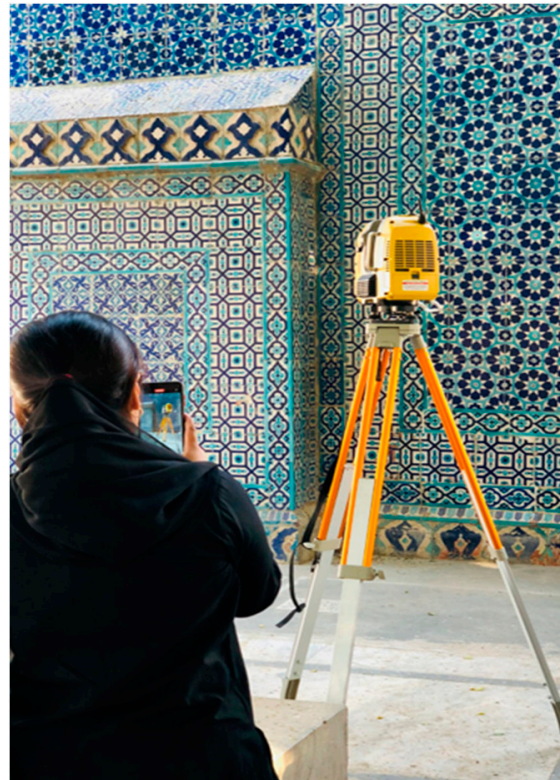
Figure 5. 3D laser scanning instrument.
