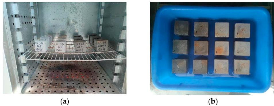
**Figure 4.** Treatment of water absorption test specimens. (a) Drying of cement mortar specimens; (b) Immersion of cement mortar specimens.
