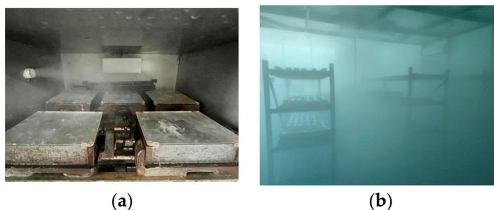
Figure 3. Curing of cement mortar specimens. (a) Graphene oxide dispersion solution; (b) Nano-calcium carbonate powder.
