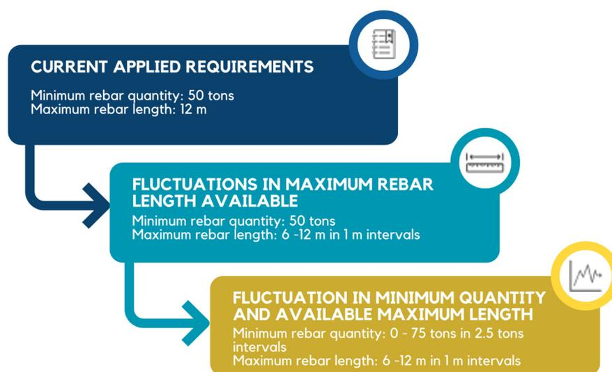
**Figure 6.** Simulation scenarios regarding the special-length rebar order within the near-zero rebar.
