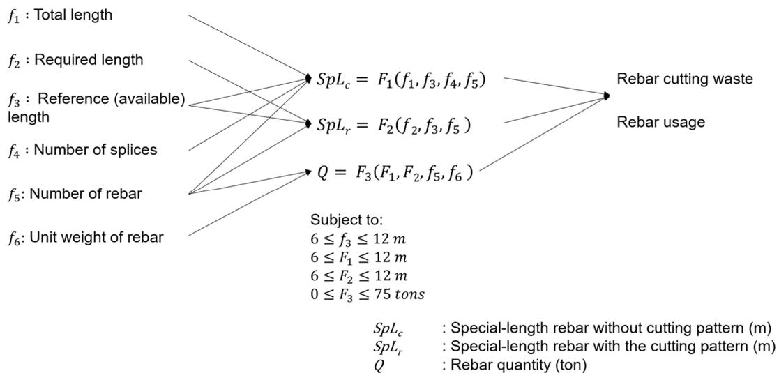
Figure 4. Optimization model (adapted and modified from [34]).
