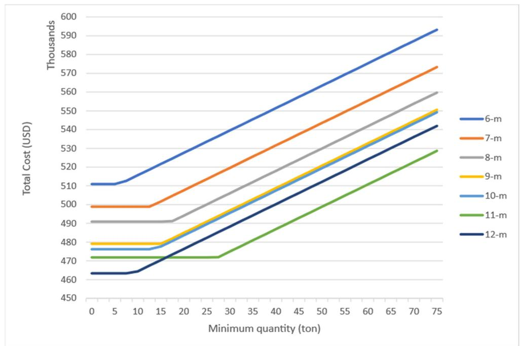
Figure 10. Simulated total reinforcement cost of columns.
