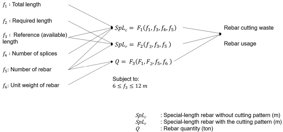
Figure 3. Simulation model (adapted and modified from [34]).
