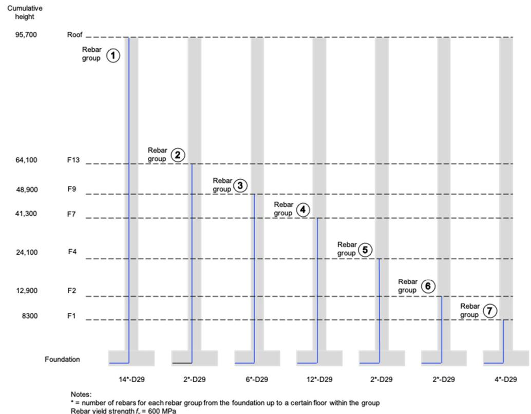
Figure 8. Rebar groups that shared similar lengths (adapted and modified from [21,40]).
