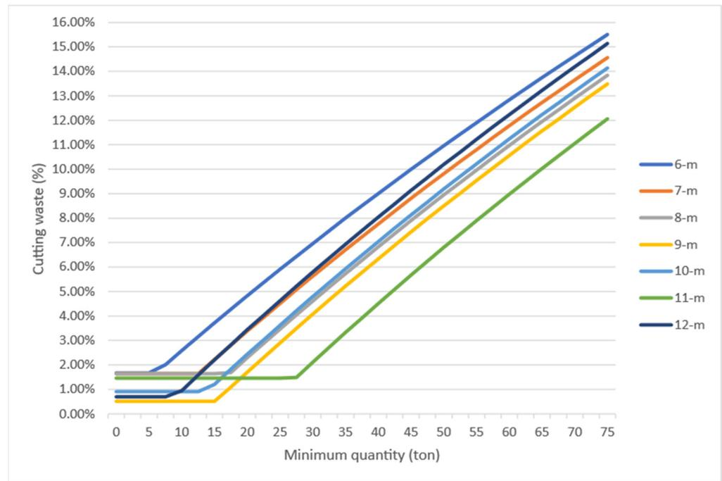
Figure 9. Simulated cutting waste generation.
