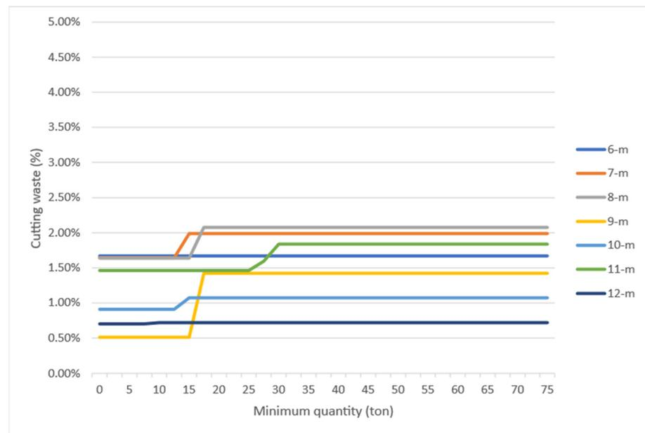
**Figure 11.** Simulated cutting waste generation following the variation of the third scenario.
