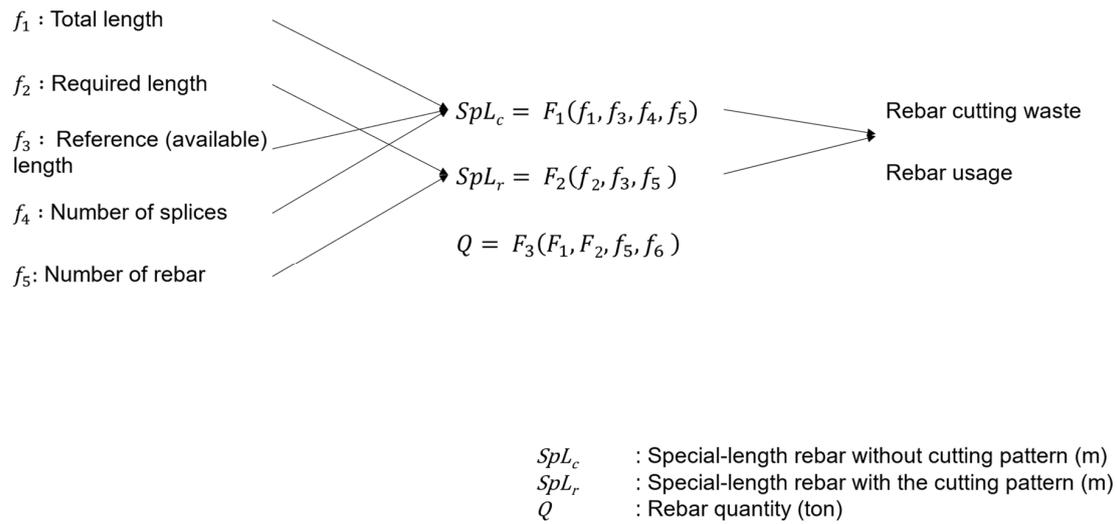
Figure 2. Generation model (adapted and modified from [34]).
