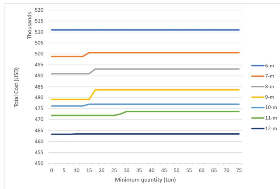
**Figure 12.** Simulated total reinforcement cost of columns following the variation of the third scenario.
