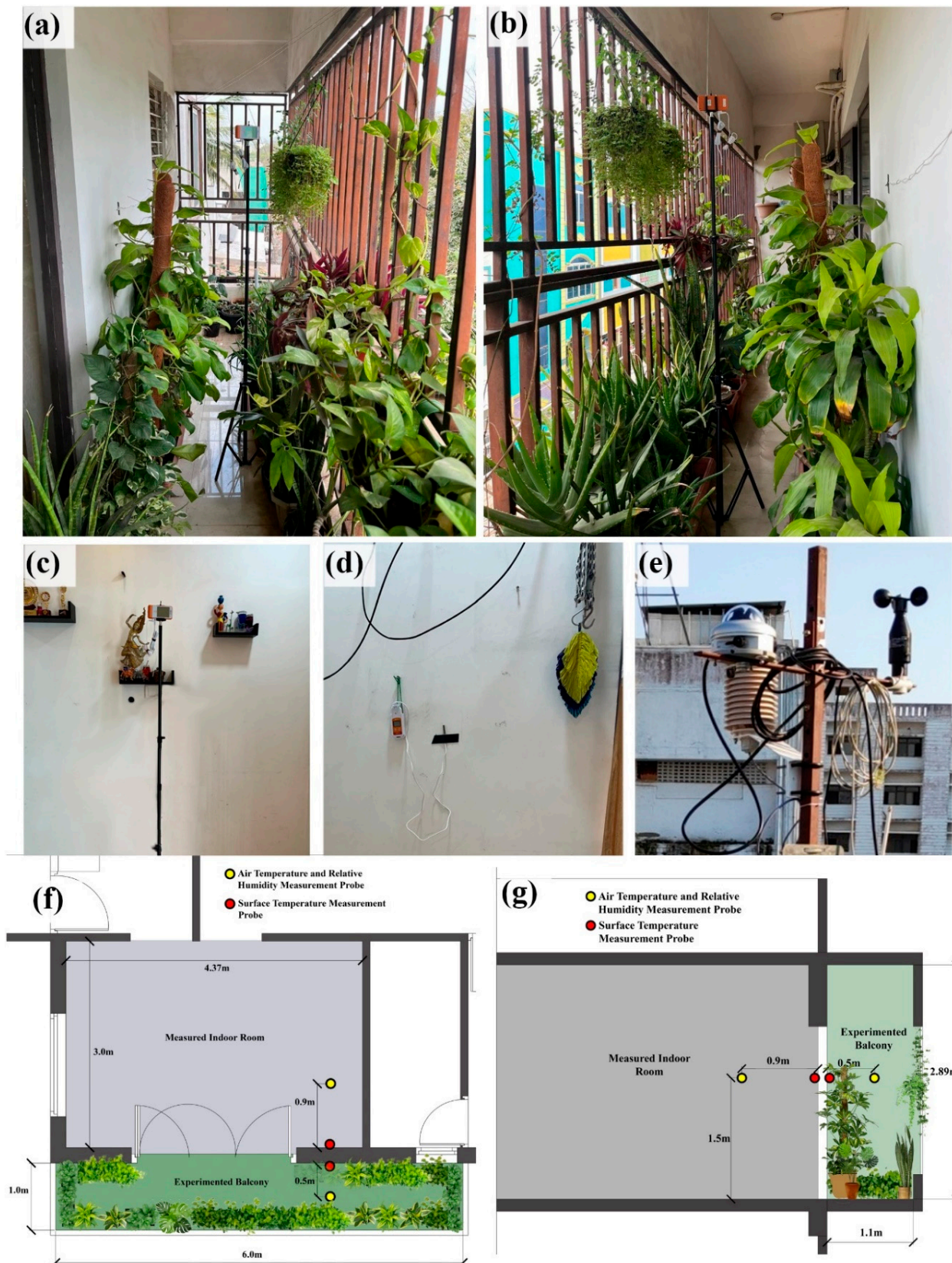
Figure 3. (a,b) Actual views of potted plants on the balcony, (c) location of indoor temperature and relative humidity (RH) sensors, (d) IST sensor, (e) weather station, including pyranometer, hygrometer, anemometer, and temperature sensor, (f,g) plan and section of the experimented balcony and room with sensors installed, respectively.
