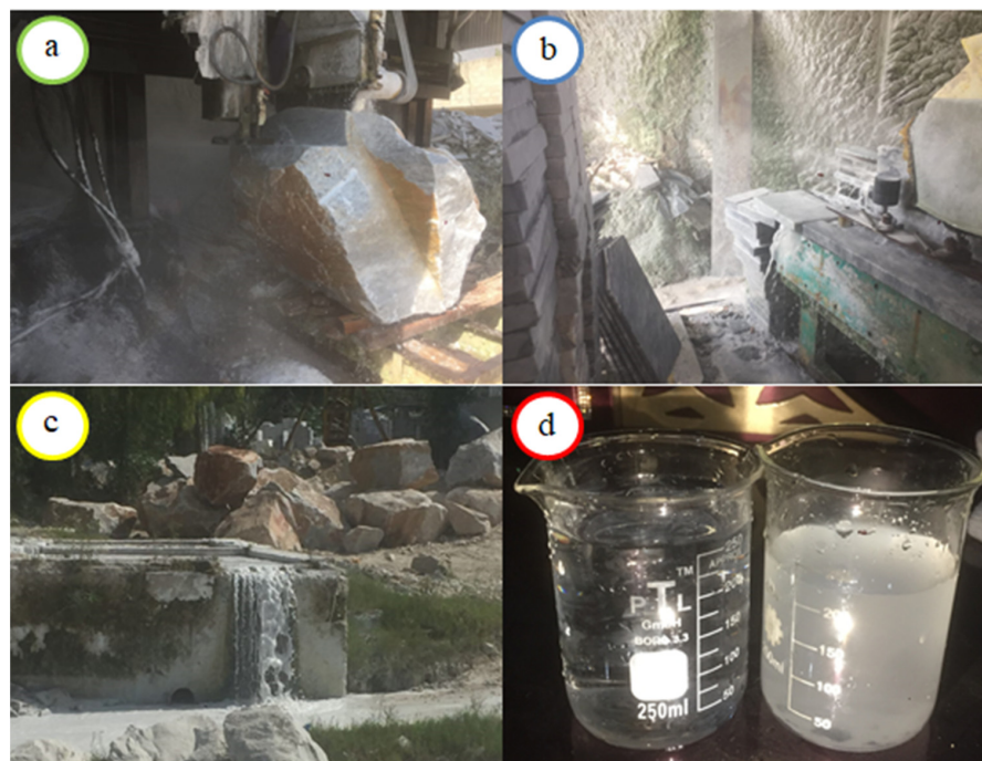
Figure 1. Photographic illustration of marble wastewater production. (a) Washing of marble rock. (b) Cutting of marble rock. (c) Marble wastewater effluence from industry. (d) Visual comparison of tap water and collected marble wastewater.
