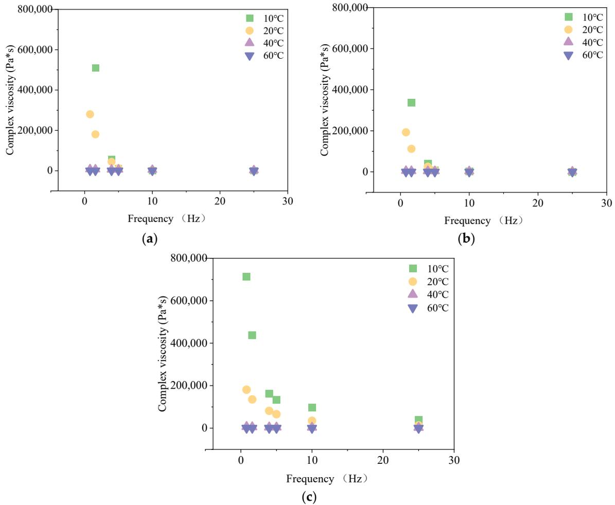
**Figure 4.** Viscosity test results of different asphalt: (a) 50# viscosity; (b) 70# viscosity; (c) SBS viscosity.
