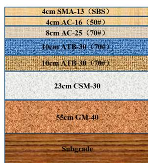
**Figure 3.** Pavement structure (AC: Asphalt Concrete; ATB: Asphalt-Treated Base; CSM: Cement-Stabilized Macadam; GM: Grading Macadam).
