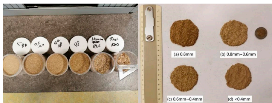
Figure 1. Appearance of reed fiber (0.8 mm, 0.6 mm to 0.8 mm, 0.4 mm to 0.6 mm, and less than 0.4 mm).
