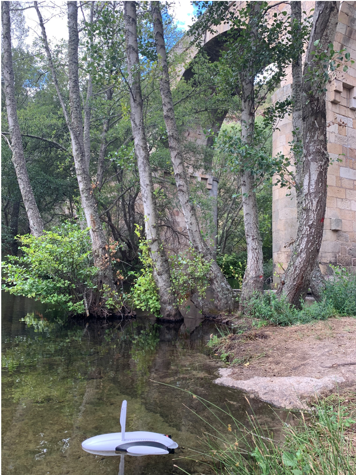
Figure 1. General view of the underwater drone used to inspect the San Lorenzo Bridge. At the time of the photo, the device was being launched towards the submerged elements of the structure for reasons of accessibility (photo by the author).
