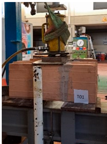
Figure 7. Setup of shear tests on triplets.
