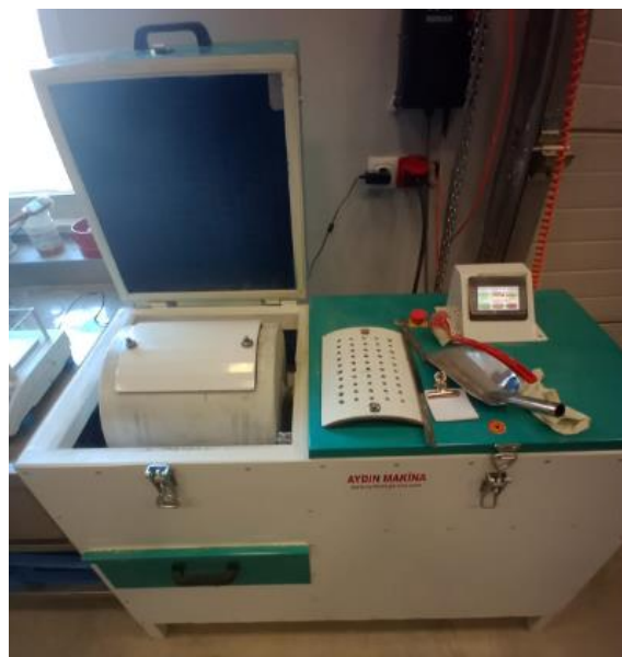
Figure 3. Laboratory-type mill used in the grinding process of cement.
