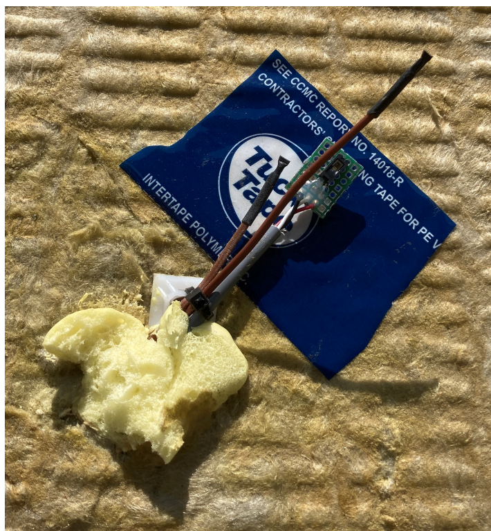
Figure 6. HIH-4000 humidity sensor and GG-T-24-SLE thermocouple type T sensors.
