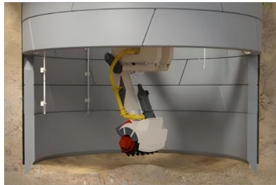
Figure 6. Shaft sinking method and schematic diagram of the sinking system.
