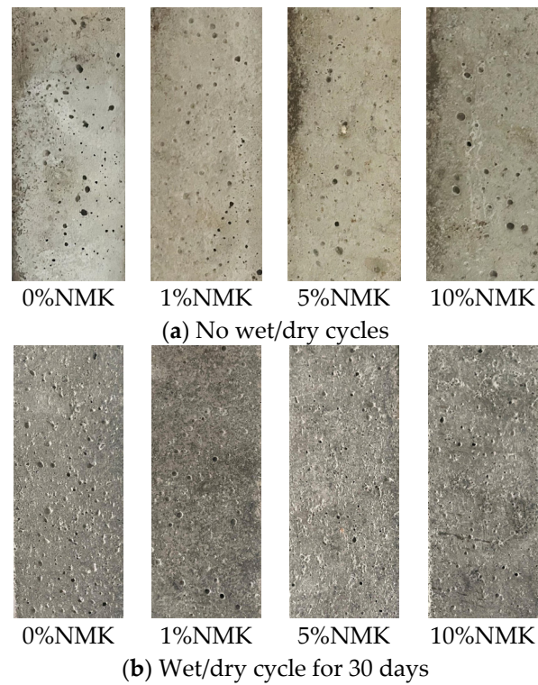
Figure 3. Changes in appearance and morphology of different nano-metakaolin without wet/dry cycling and wet/dry cycling for 30 d.
