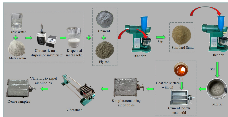
Figure 2. Preparation process of specimen.
