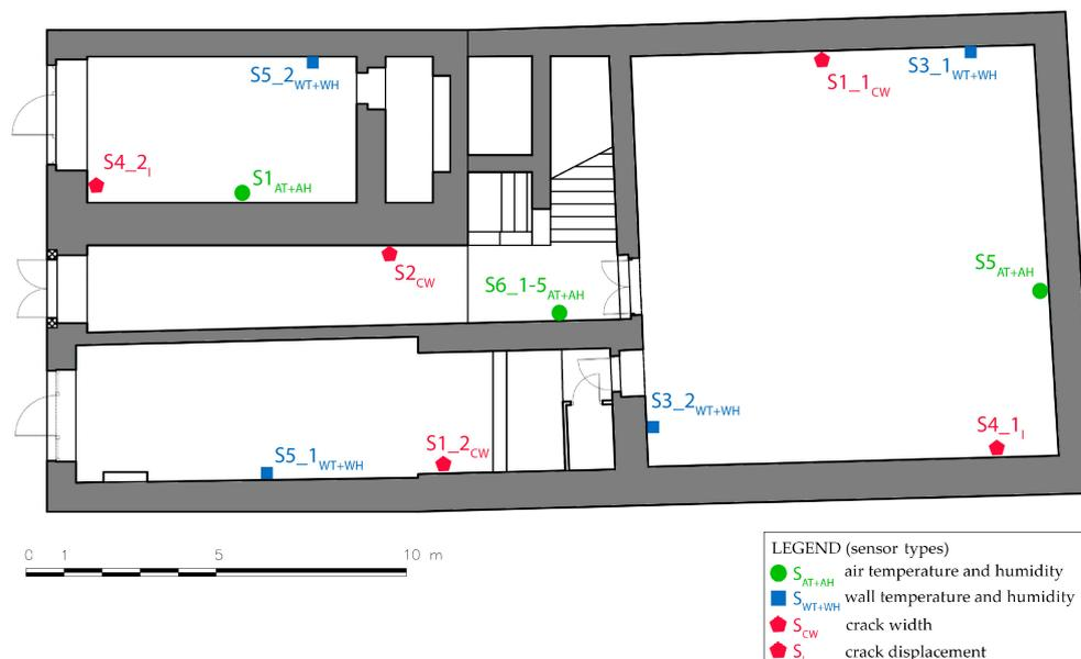
**Figure 3.** The layout and placement of the used sensors within the building.
