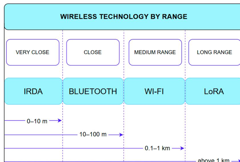
**Figure 1.** Signal propagation range in data transmission using IoT technology.
