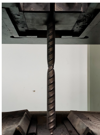
Figure 4. Failure phenomenon of steel reinforcement.
