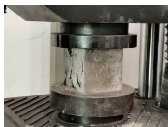
Figure 3. Failure phenomenon of cubic specimens.
