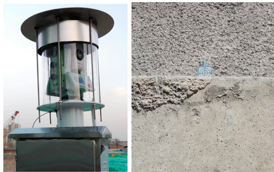
Figure 14. Automated total station and measurement target.
