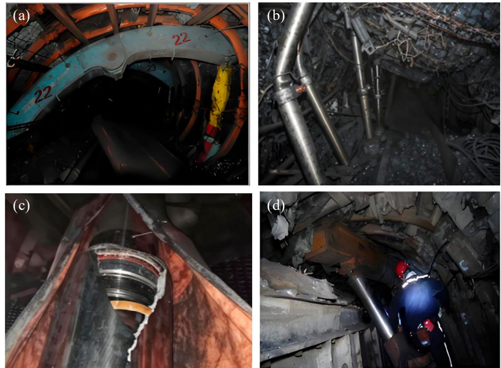
**Figure 1.** Impact destruction of hydraulic supports. (a) Support failure. (b) Column bend. (c) Cylinder burst. (d) Beam failure.
