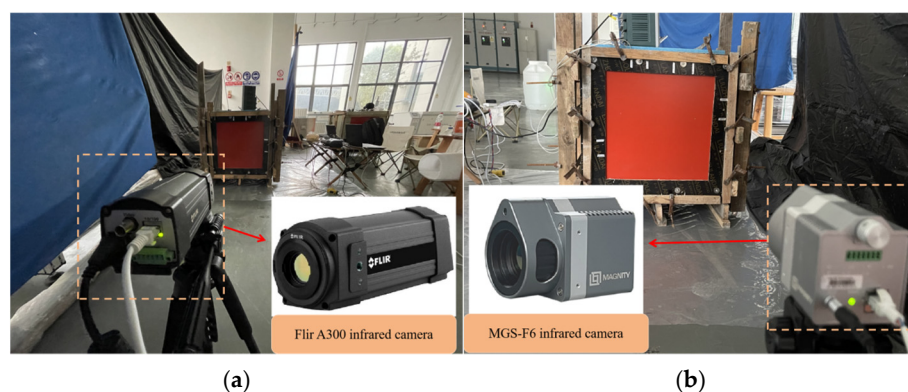
Figure 8. Infrared imaging setup: (a) FLIR A300; (b) MGS-F6.
