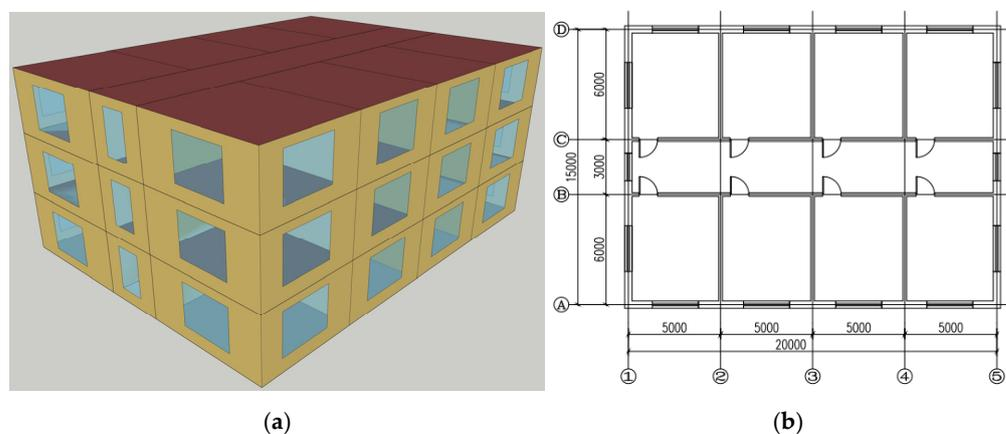
**Figure 2.** Model drawings and floor plans of typical office buildings. (a) SketchUp model diagram; (b) CAD plan of the building.
