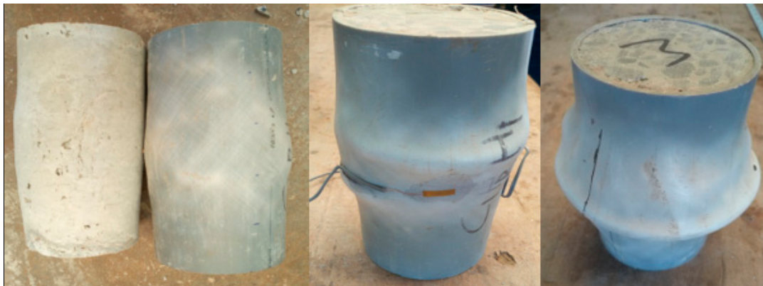
Figure 8. Drum Type Failure.
