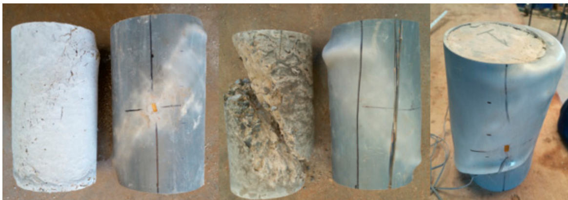
Figure 9. Shear Type Failure.
