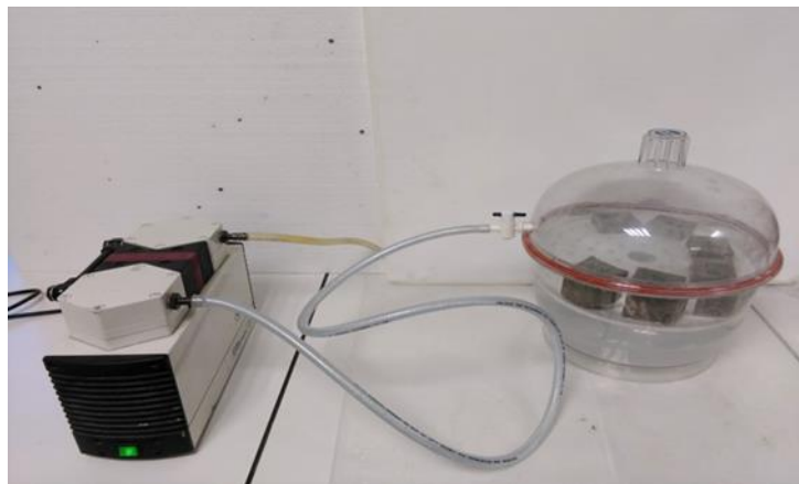
Figure 4. Vacuum specimen saturation.
