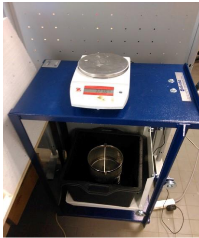
Figure 5. Hydrostatic weighing instrument.
