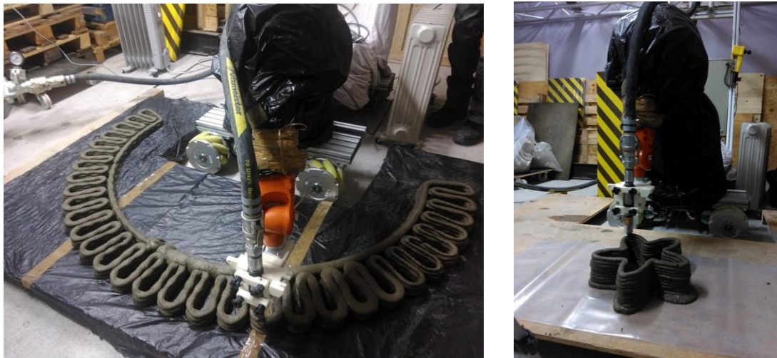
Figure 3. Images from the second 3D printing campaign that resulted in the MCR20-01-17 samples. (French Project MATRICE [40]).
