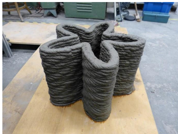
Figure 2. Image from the first 3D printing campaign that resulted in the MC14-10-16 samples. (French Project MATRICE [40]).
