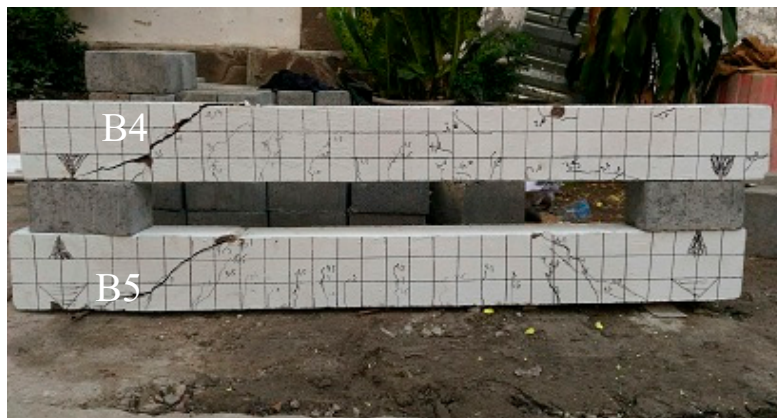
Figure 8. Crack pattern of the series II test (B4 and B5).
