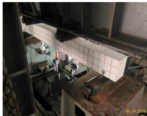
Figure 6. Loading test of geopolymer concrete beam (GCB).
