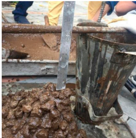
Figure 2. Slump test of the geopolymer concrete mix.
