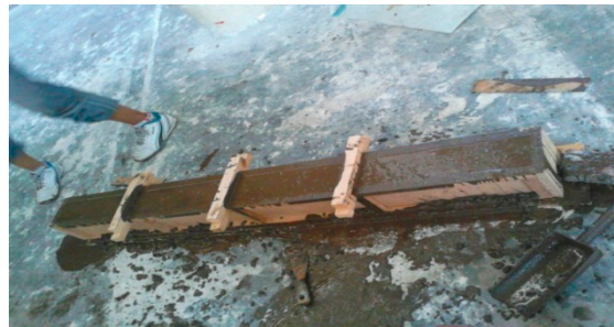
Figure 3. The geopolymer concrete beam after casting.
