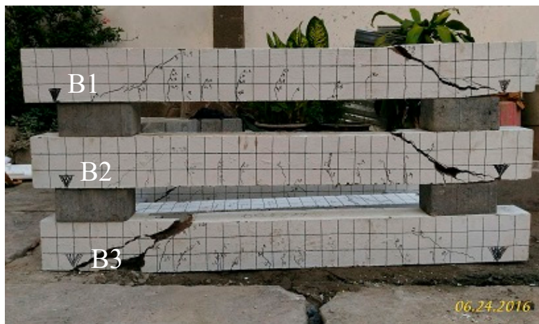
Figure 7. Crack pattern of the series I test (B1, B2, and B3).
