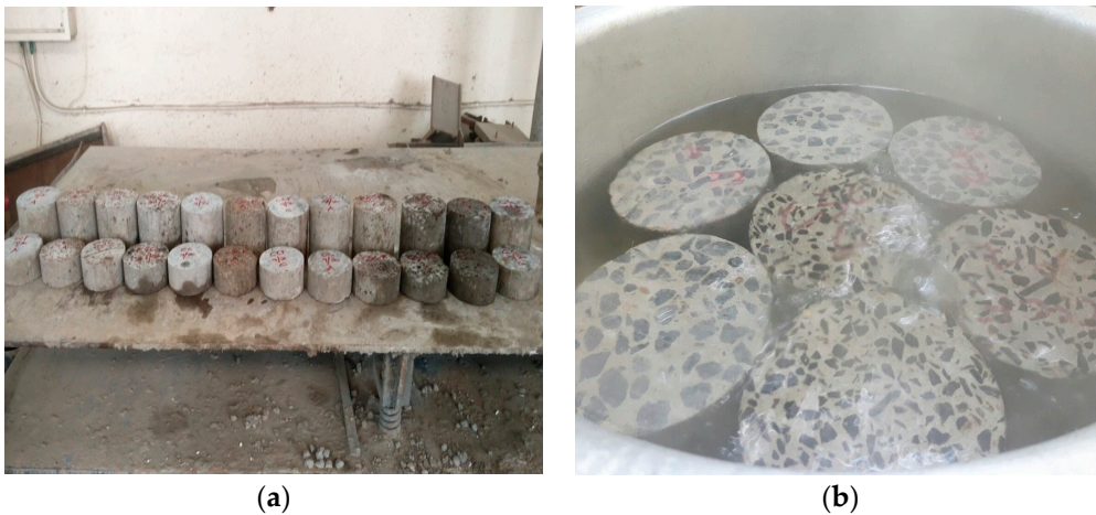
Figure 2. (a) Center core cut specimens (b) specimens under boiling.
