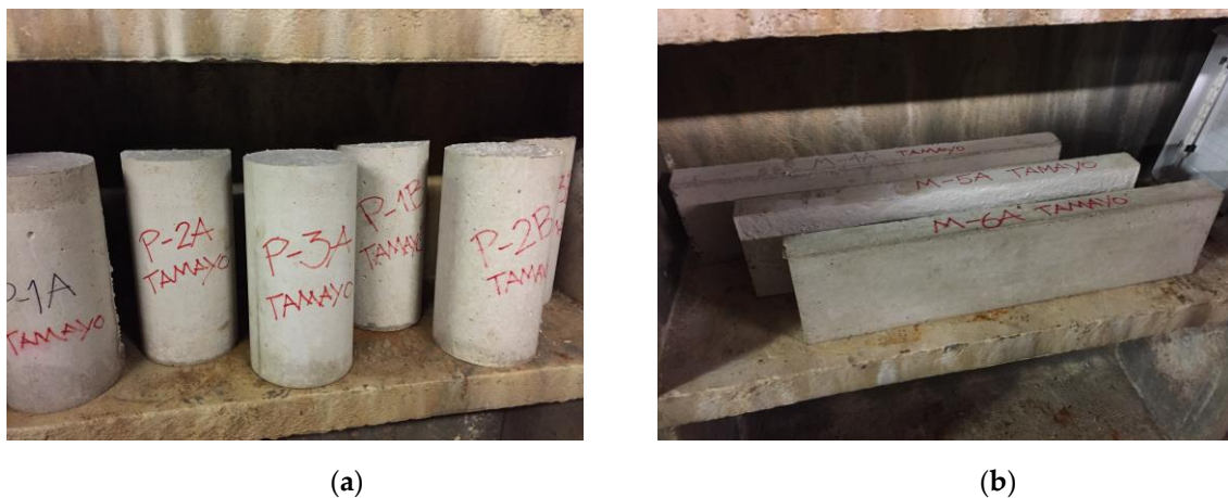
Figure 4. Curing process. (a) Cylindrical specimens; (b) Rectangular specimens.
