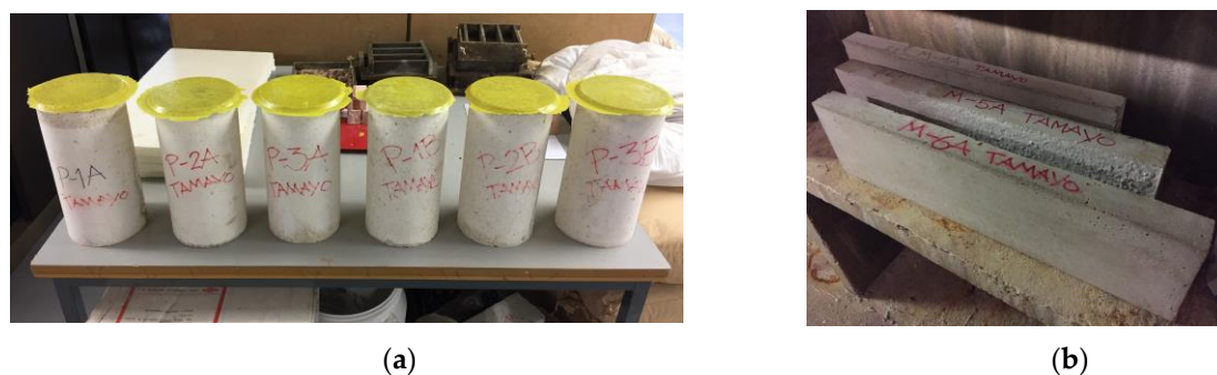
Figure 5. Final preparation of specimens. (a) Cylindrical specimens; (b) Rectangular specimens.
