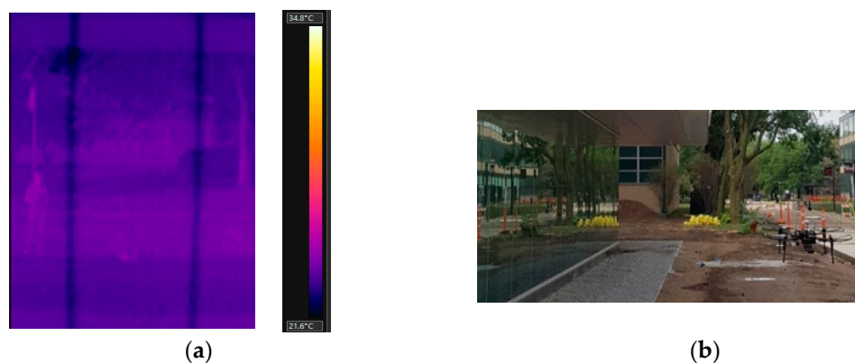
Figure 6. Collecting noncontact temperature from the building envelope using UAV. (a) Frame of thermal image; and (b) data collection using UAV.
