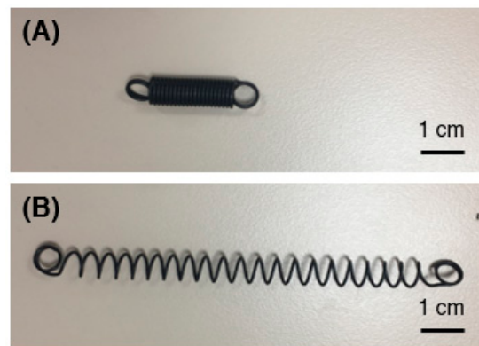
Figure 1. (A) Original shape of SMA spring. (B) Shape of SMA spring after deformation.
