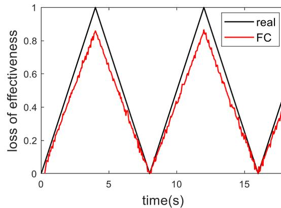
**Figure 4.** Actuator effectiveness reconstruction result of the observer.
